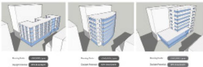
The above illustrates the non-linear outcomes and complexity involved in building physics analysis. The cheapest building to run offered the most daylight potential.
